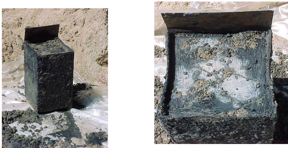
Figure 1. A view of a container with glass K-26 (left) and the glass surface interfacing with backfill (right).
